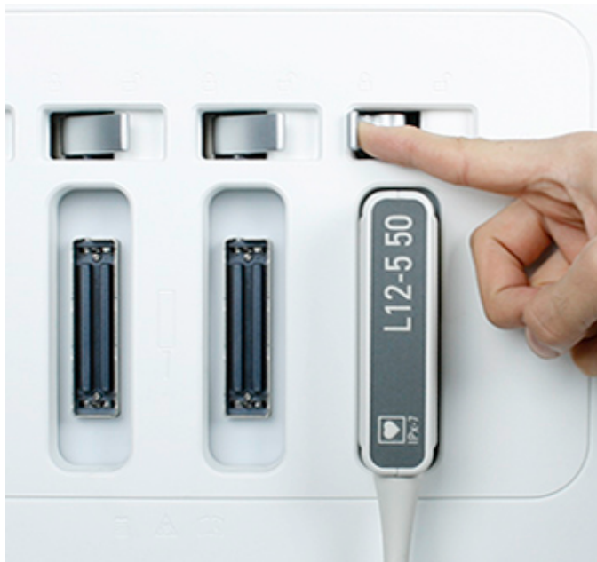
Connecting a Transducer to the System
