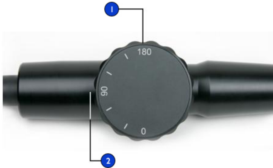
Rotating the S8-3t Imaging Array
