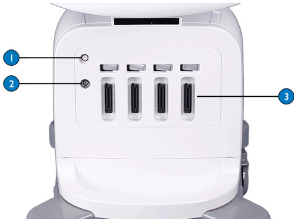
Transducer and Physio (ECG) Receptacles
